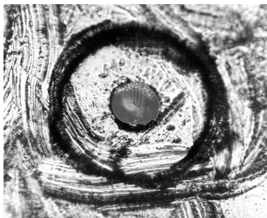
Figure 1-6. Damage from improper cleaning.
